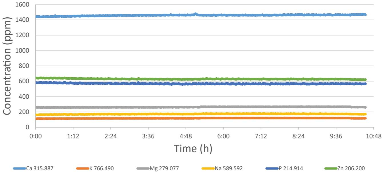
**Figure 5.** SampleSense Oil with 4DXCi autosampler using controlled gas infusion mixing for 23 elements measured over 1764 used motor oil samples in 10 hours and 30 minutes. Stability of six elements with higher concentrations shown above. Lower concentration elements showed similar stability.
