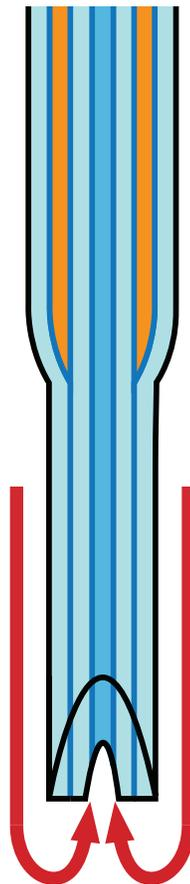
**Figure 2.** The figure above shows the V-shaped tapered tip probe. The figure shows the side view, where the cutouts reduce the oil-coated surface area and allows the vacuum to efficiently remove excess droplets.
