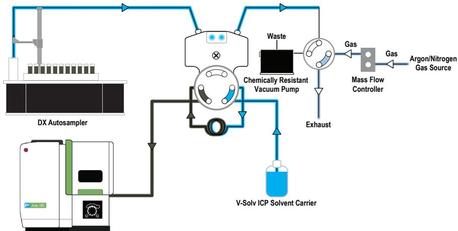
**Figure 1.** SampleSense Oil Controlled Mixing Diagram: (1) Gas infusion valve switches to allow gas flow through SampleSense valve and out the probe. Probe moves into the sample and mixes by gas infusion. (2) With the sample mixed, the gas infusion valve switches and vacuum loading of the loop begins. (3) Once the loop is filled and the sample is sensed, the SampleSense valve switches and sends the sample to the instrument while uptake path is rinsed.
