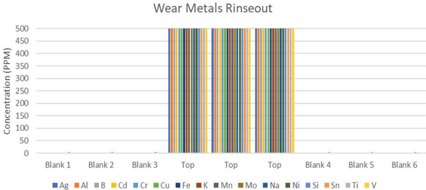
**Figure 6.** 500x washout for all wear metals.
